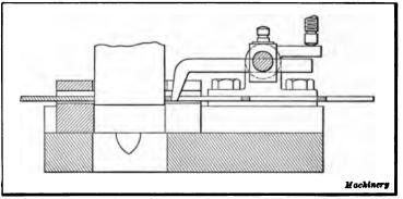
Fig. 33. Simple Latch Form of Stop
